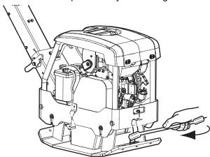
Check the screws and nuts on the safety straps, if necessary tighten or replace.
