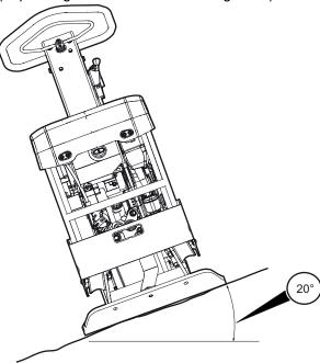
◆ The tilting angle is measured on a hard level surface with the machine stationary. Vibration switched OFF and all tanks full.
