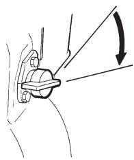
4. Pull out the starter rope until it resists. Release the handle so the starter rope goes back again, and then pull the starter rope until the engine starts.
