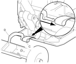
4. Lock the handle (E) and tilt the machine forwards. Fold the trolley (D) in under the bottom plate (F).
